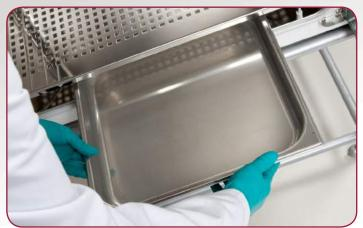
Water Tray - separate heating element for increased control of humidity
